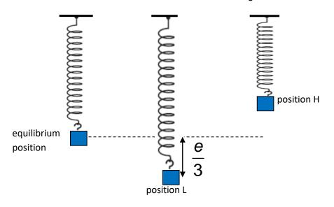
When the mass is released, it performs simple harmonic oscillations between positions L and H with angular frequency  $\omega$ . The displacement from equilibrium is given by the equation
